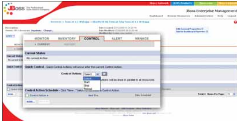
The Administration Module allows you to perform control actions such as start, stop, and re-start on a single application or across an enterprise cluster.
